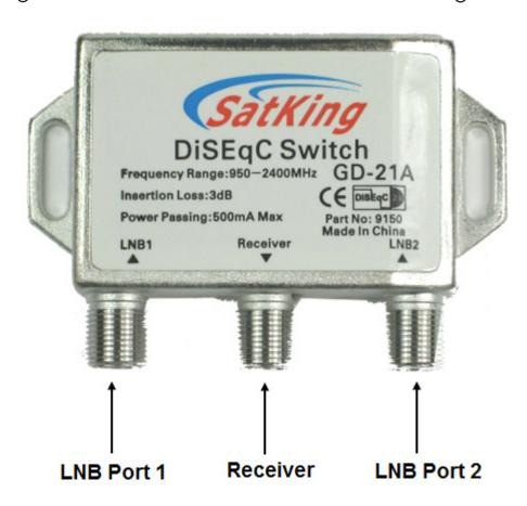
This DiSEqC switch is to connect two dishes into one receiver. Simply go into LNB setup in your receiver and for the first sateelite select port 1 and for the second satellite select port 2. No power injector is required for this DiSEqC switch as the power is provided by the satellite receiver.
